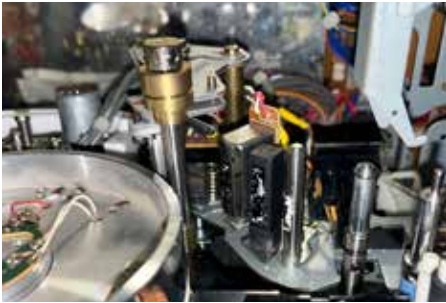
Magnetic tape residue in MARMIA's U-matic deck. Image courtesy of MARMIA.
